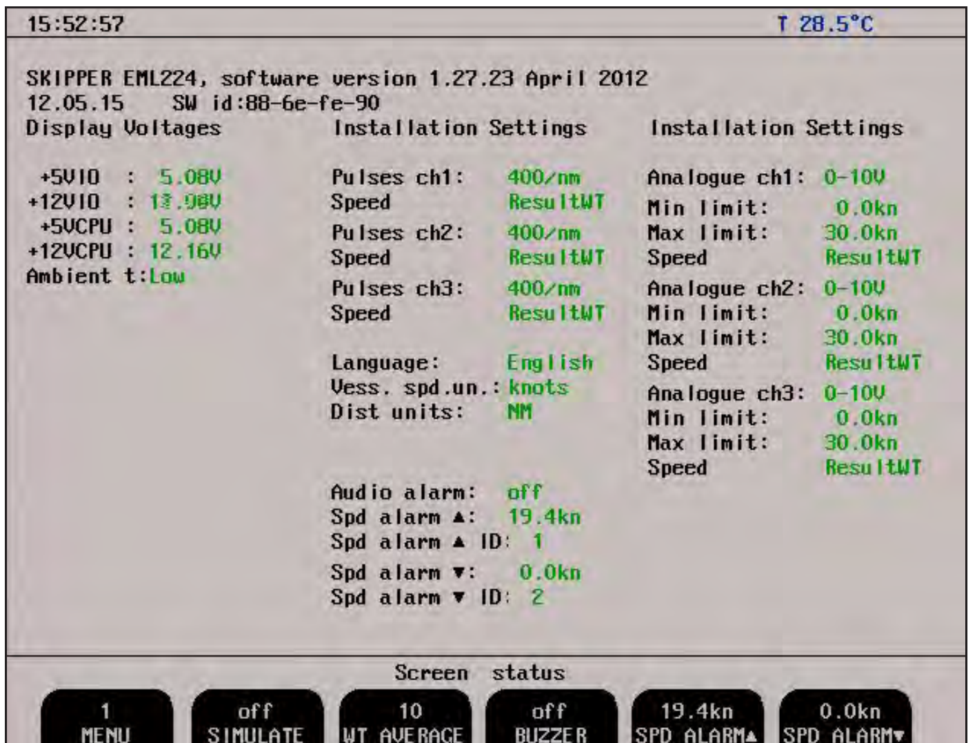
Fig. 8.1 Typical contents of status screen
